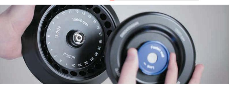
DLAB hematocrit centrifuge with AC24P hematocrit rotor is used for determination of volume fractions of erythrocytes in blood for diagnostic purposes and doping tests. Also it is used for the photometric determination of bilirubin content in neonate blood samples. Hematocrit centrifuge with A24-2P tube rotor, can be used for extraction of DNA and RNA.
